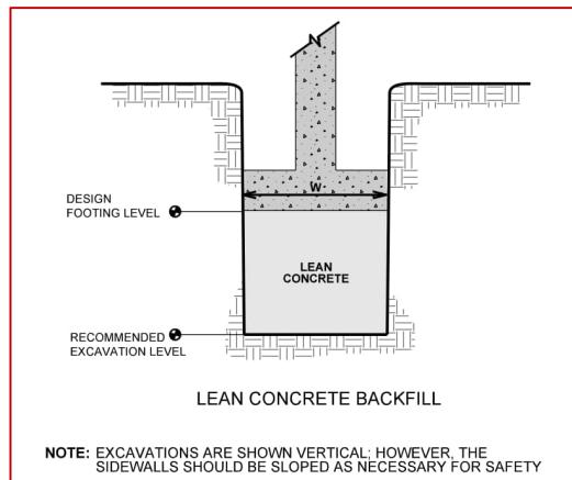
As an alternative, the footings could also bear on properly compacted structural backfill extending down to the suitable soils. Over-excavation for structural fill placement below footings should be conducted as shown below. The over-excavation should be backfilled up to the footing base elevation, with structural fill placed, as recommended in the [Earthwork](#) section.
